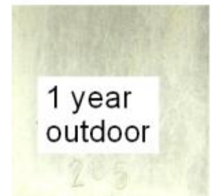
Corrosion products of EN AW-6060-T6
